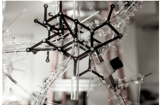
Figure 6. A detailed view of the node which houses a junction split and a gravity-fed solenoid valve
